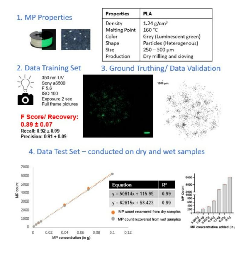
Developed protocol has a recovery rate of 89%
