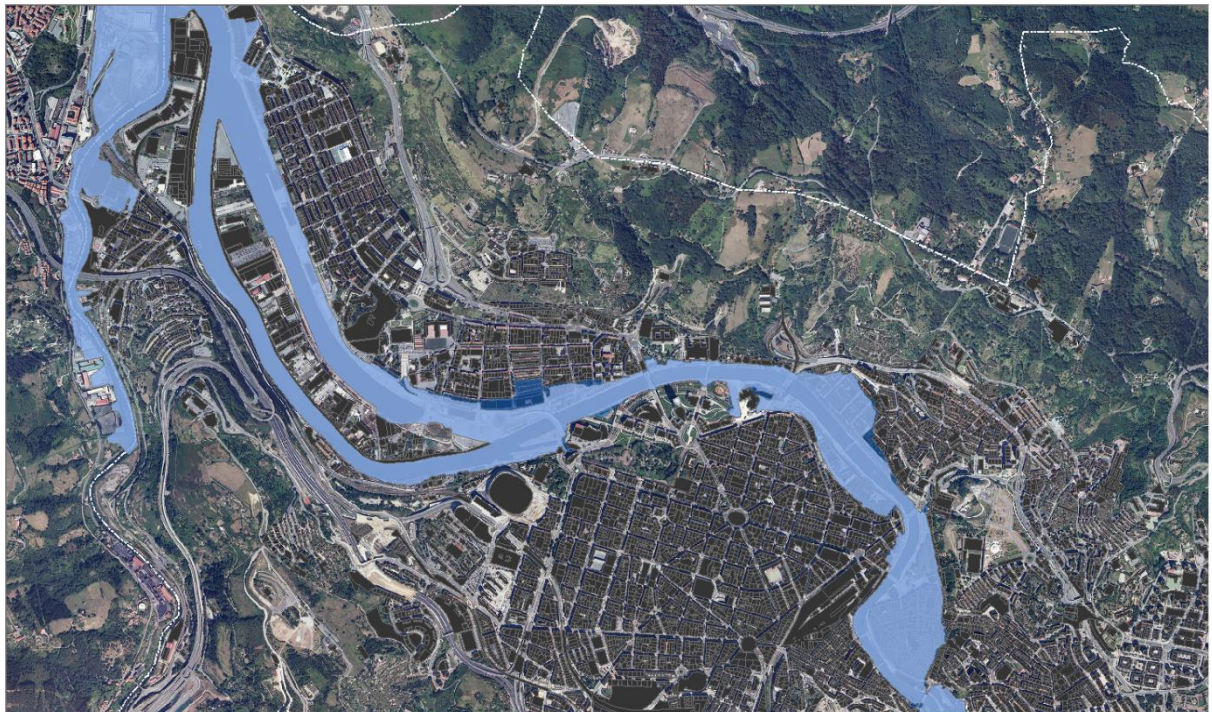
Figure 2. The 100-year return period flood risk map. In dark blue the areas affected without the opening of the canal, while the light blue area represents the potentially flooded areas once the canal has been built.
