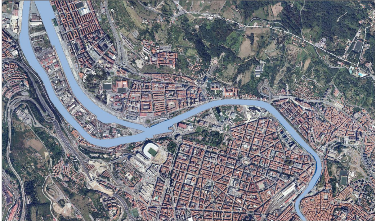
Figure 1. The 10-year return period flood risk map. In dark blue the areas affected without the opening of the canal, while the light blue area represents the potentially flooded areas once the canal has been built.
