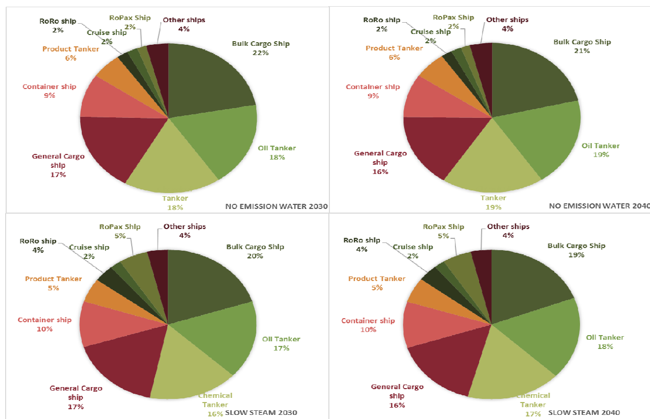
Figure 13: Copper emissions by ship types for scenarios of no-water emission and slow steaming
