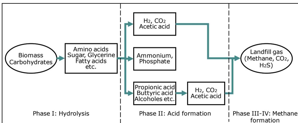
Figure 6: Biodegradation of landfilled waste (Bilitewski et al. 2000)
