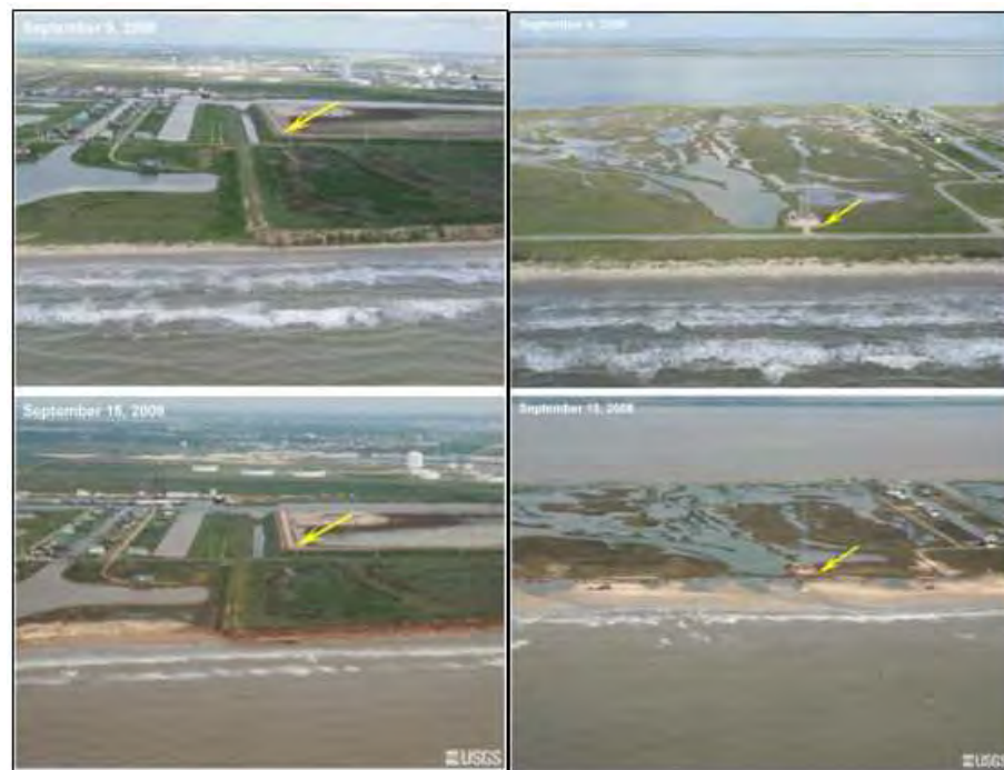
Figure 7.54 Dune erosion at location 1 of Figure 7.53 (left) and overwash of coastal road at location 2 of Figure 7.53 (right)(Source: Doran et al., 2008).
