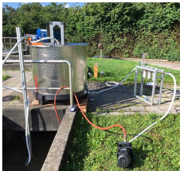
A stainless steel filter cascade is suitable for concentrating a large sample volume.
