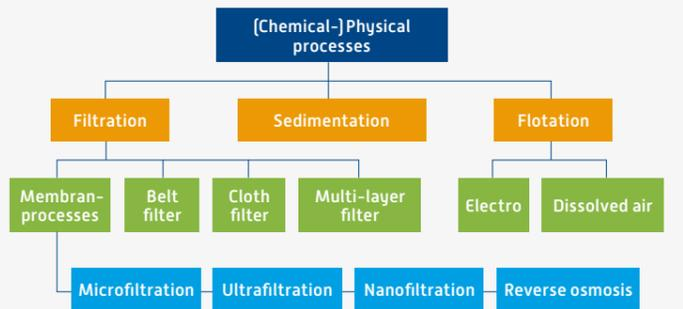
Identification of input pathways has shown that microplastics can enter wastewater along the complete value chain (production - processing - shipping). Filtration, flotation and sedimentation processes are best suited to removing them from wastewater. The efficiency of these processes could be significantly improved by specially developed flocculants.
