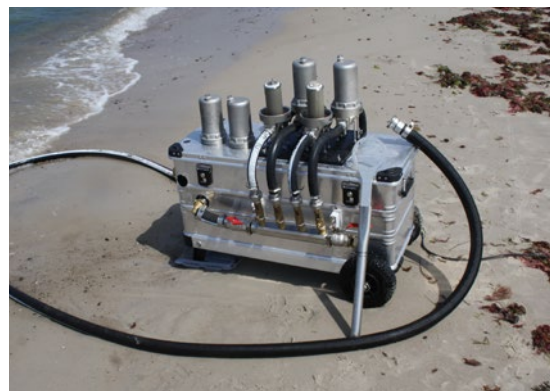
Fig. 3: The 'Rocket' device, developed specifically for the sampling of microplastics, during a test sampling at the Baltic Sea.
