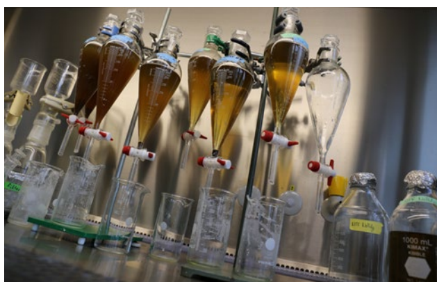
Fig. 2: Density separation of the light components (plastic/organics) from heavy sediments. Microplastic analyses from environmental samples are very laborious and time-consuming. Several months pass from sample collection to result.
