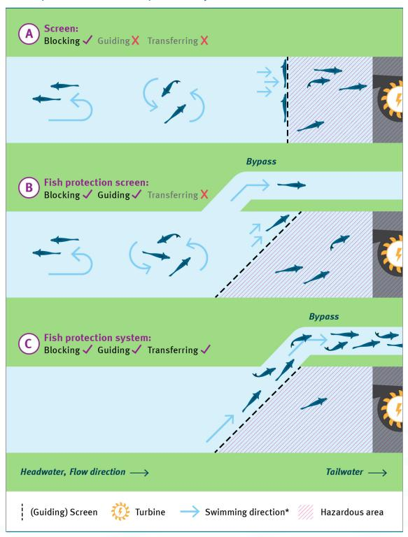
A fish protection system always consists of a fish protection screen and a bypass, designed as a functional unit.
