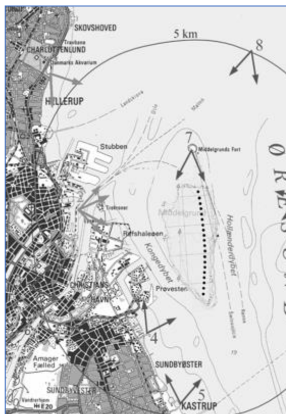
Figure 8 The position of the 20 wind turbines within the 6-meter water depth contour
