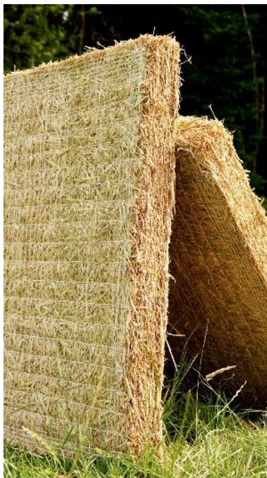
Figure 4 Example of COPANO's straw panels
