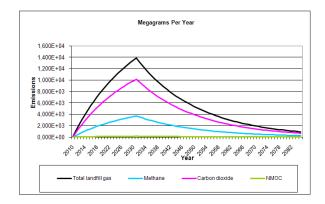
Total methane emissions are assessed at 170.164.940  $m^3$  of methane emissions over the whole lifespan of the landfill plus its after-phase. This can be translated in a ratio of 170  $m^3$ /tonne landfilled MSW.
